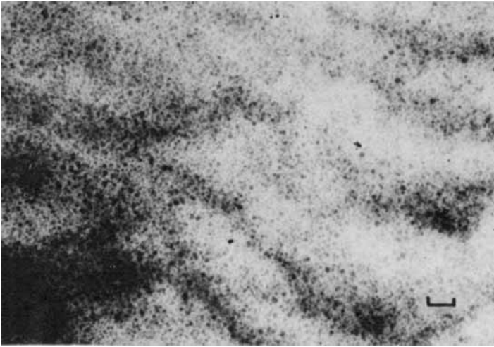
Fig. 3. Electron micrograph of the semi-1-IPN containing 40% by weight of polyurethane. Scale mark represents 1000 nm.
